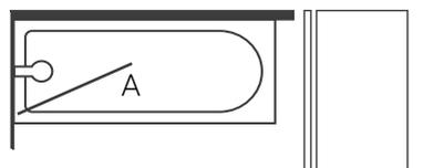
A: Moving Panels (screen width when folded into the bath 712mm)
