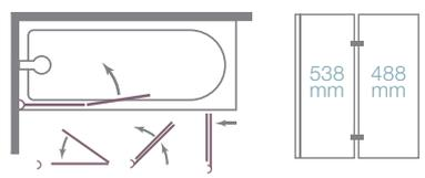
Door Swing: 180 degree radius of screen swing inwards and outwards
