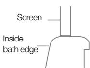
Please ensure product is fitted with panel positioned in line with the inside bath edge.
